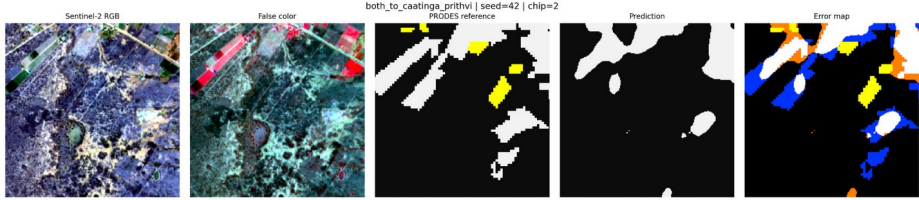
Fig. 6. Qualitative example of Both-to-Caatinga segmentation for Prithvi-EO on the same Caatinga target chip. Including Caatinga samples during training mitigates the all-positive collapse observed in Amazon-to-Caatinga transfer and produces a spatially structured prediction, although boundary and localized classification errors remain. In the error map, white = true positive, black = true negative, orange = false positive, blue = false negative, and yellow = ignored.
